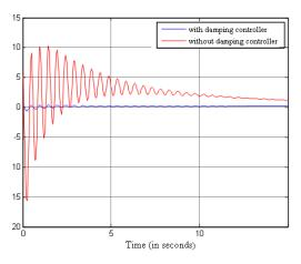
Fig.7 The UPFC controller having load Pe=1 with and without damping controller  $m_E$
