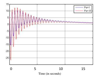
Fig.9 Dynamic response of mE damping controller with wide variation in loading
