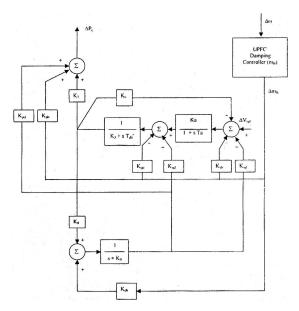
Fig 5. Transfer function of the system relating component of electrical power ( $\Delta Pe$ ) produced by damping controller ( $m_B$ ).
