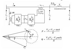
Fig:2 Implementation of the unified power flow controller
