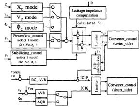
Fig 3.Control scheme of UPFC Model
